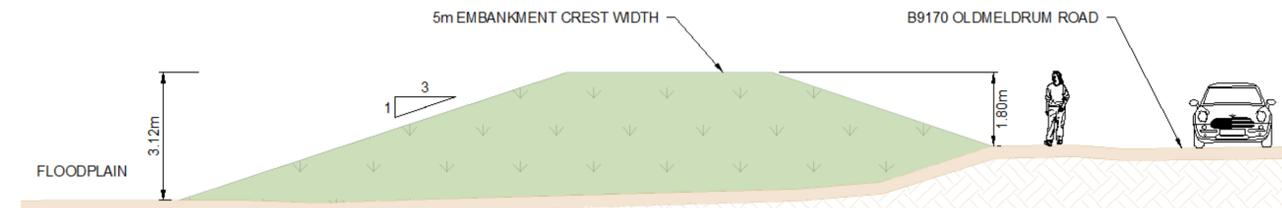
**Section A-A: Oldmeldrum Road embankment cross section (sizing for 200 year plus climate change)**
