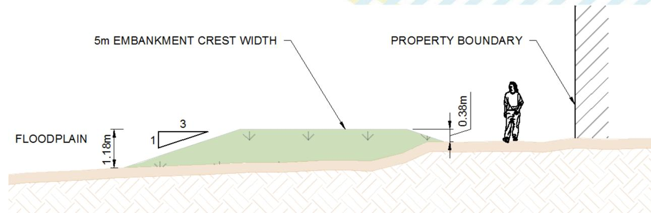
**Section B-B: "Gauld's Gas" embankment cross section (sizing for 200 year plus climate change)**
