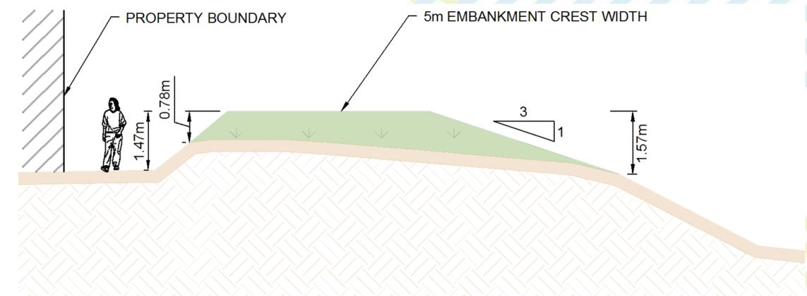
**Section C-C: Canal embankment cross section (sizing for 200 year plus climate change)**
