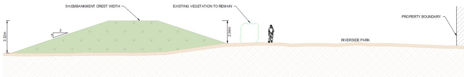
**Section D-D: Davidson Field embankment cross section (sizing for 200 year plus climate change)**
