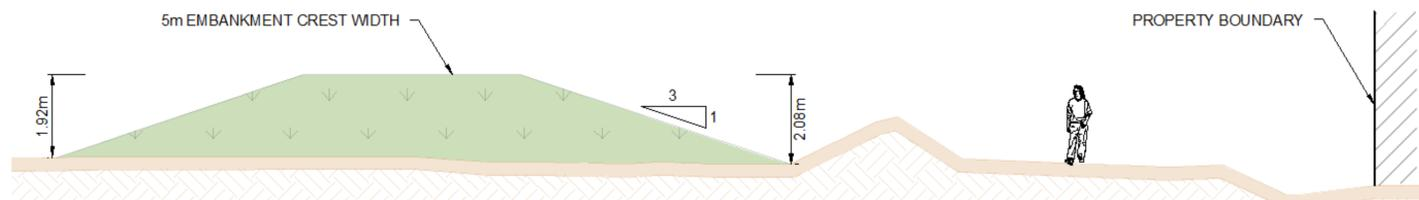
**Section E-E: Scottish Water embankment cross section (sizing for 200 year plus climate change)**
